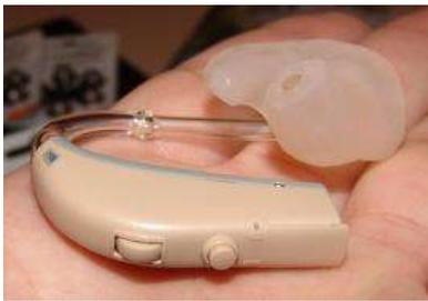
*A behind-the-ear (BTE) hearing aid in the palm of a hand. The image shows the main shell section of the aid, which is placed behind the ear, and the tube connecting the main shell with the ear-mold, which is inserted into the ear canal. The hearing aid is designed to match skin color.*
