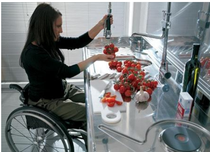
Figure 32 The photograph shows an accessible kitchen worktop. All the elements are within the easy reach of both sitting and standing users ( http://www.tuvie.com/hability-easyfood-and-valcucine/ ).
