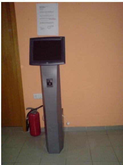
Figure 21 - The photograph shows a Studomat, in front of which enough maneuvering space is provided, but the screen is outside the visual reach of a student in a wheelchair.
