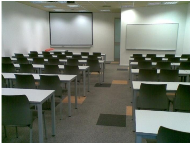
Figure 31 - The photograph shows a classroom designed in such a way that the entrance is on the same level as the floor, and there is a sufficiently wide aisle between the desks to allow barrier-free passage.
