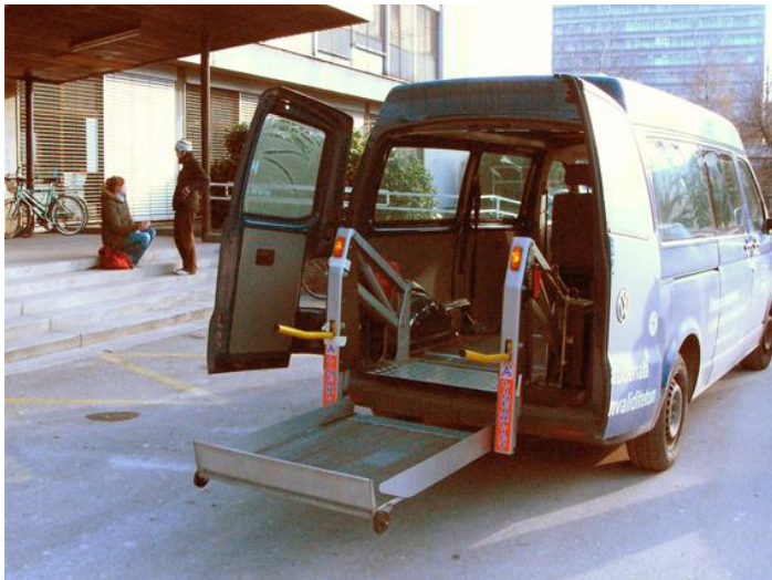
Figure 27 - The photograph shows a van for the transportation of students with disabilities. A folding vertical wheelchair lift can be seen, and – inside the vehicle – a safety belt for fastening a wheelchair.
