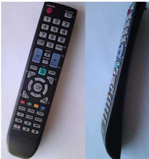
Figure 30 - The photograph shows a TV remote control which is ergonomically shaped, with clear and noticeable buttons containing text, symbols and tactile signs for the blind and visually impaired.
