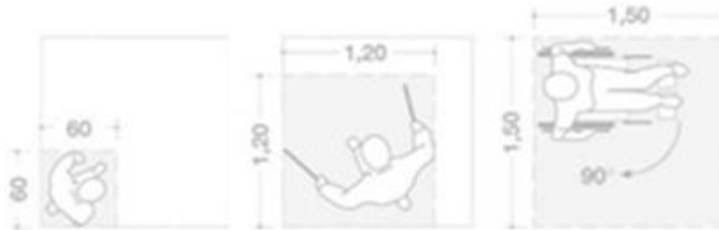
Figure 12 - The illustration shows different dimensions of maneuvering space, which depend on one's requirements ( http://www.gradimo.hr/3573.aspx ).
