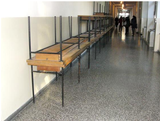
Figure 2 - An example of bad practice: The photograph shows horizontal barriers (desks) in a university hallway that present obstacles and hinder the movement of blind and visually impaired students.
