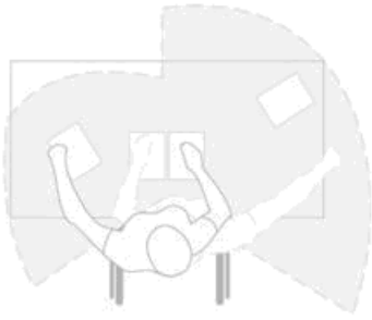
Figure 8 - The illustration shows the horizontal area of active reach of students in wheelchairs ( http://www.gradimo.hr/3573.aspx ).
