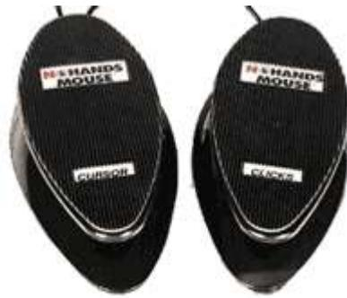
Figure 7. Foot controlled computer mouse (taken from [http://www.spd.org.sg/programmes/assistive/atc\\_alternativemouse.html](http://www.spd.org.sg/programmes/assistive/atc_alternativemouse.html))
