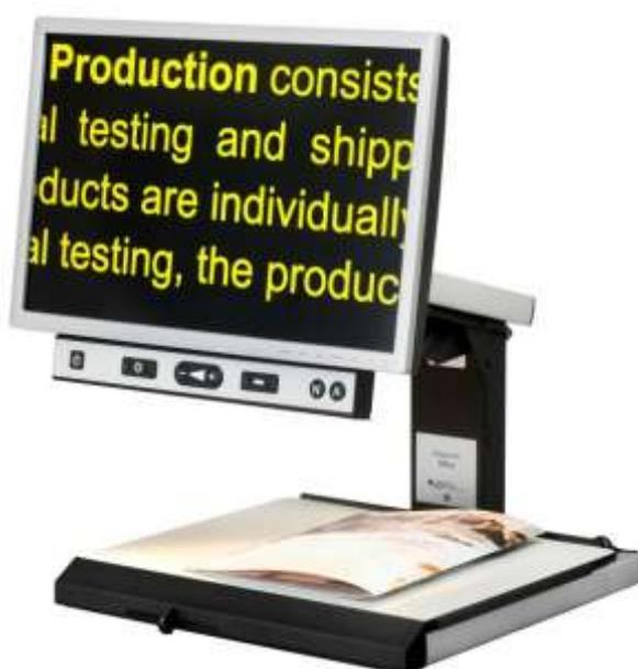
Figure 3. Video magnifier or *Closed Circuit Television (CCTV)* (taken from <http://www.savez-slijepih.hr>)
