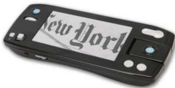
Figure 2. Portable electronic magnifier (taken from <http://www.savez-slijepih.hr>)
