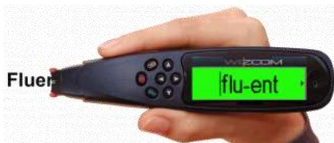
Figure 9. Reading Pen, a device adapted for people with dyslexia
