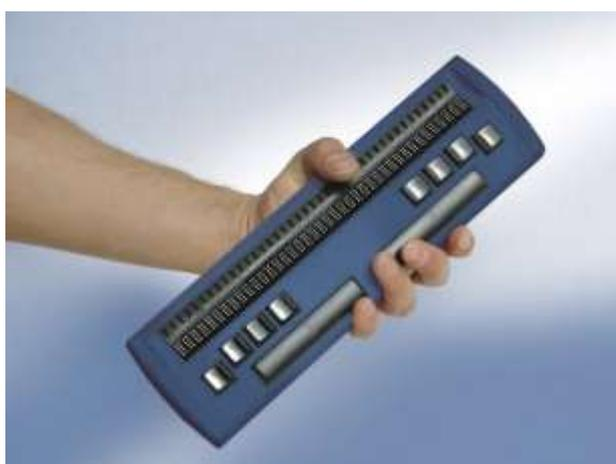
Figure 1. Braille line (taken from <http://www.savez-slijepih.hr>)
