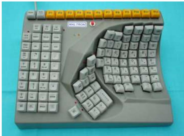
Figure 8. Alternative keyboard adapted for one-handed typing (taken from [http://www.spd.org.sg/programmes/assistive/atc\\_alternativekeyboards.html](http://www.spd.org.sg/programmes/assistive/atc_alternativekeyboards.html))
